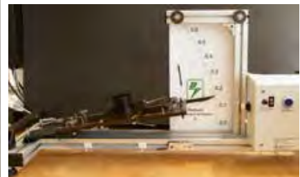
Measurement of the coefficient of friction
